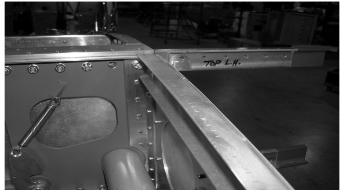
The photo above shows the outboard wing fitting going into the center section. (Ends with red tape are on the inside of the wings.)
