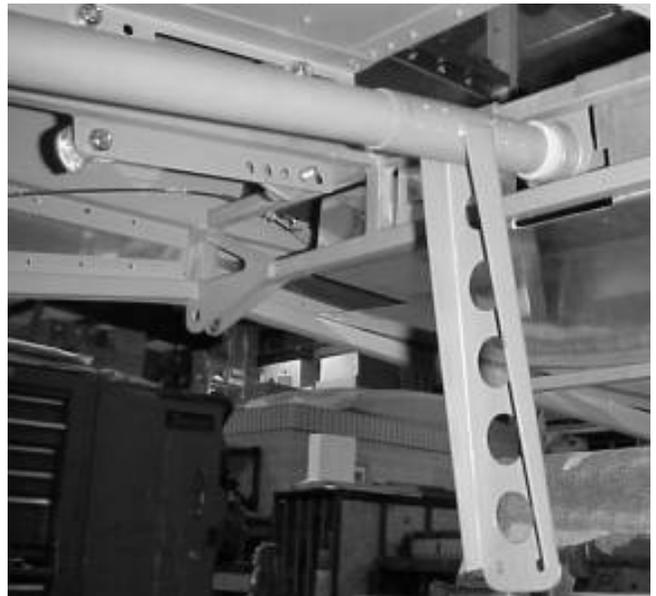
Stick assembly as viewed from under the front seat looking forward from the right side. Let the aileron driver swing freely until the wings and aileron push/pull tubes are installed.
