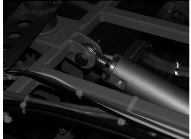
Looking forward and down from the left side of the fuselage. Shows elevator bellcrank (dark green) and tailwheel hydraulic cylinder.
